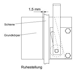
The knurled braking roller shall be in full contact with the guide rail blade.
