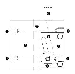
The safety gear must be mounted in pairs. They should be recessed into the structure, otherwise a limit stop shall be provided.
